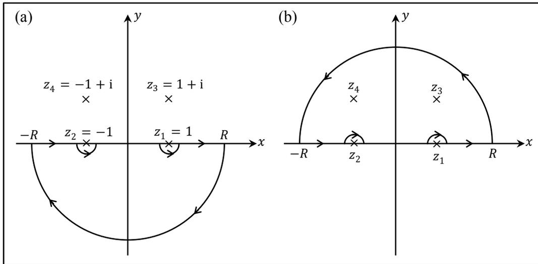
In Fig.(a) the contour is closed in the lower-half of the  $z$ -plane. The closed contour does *not* contain any poles and, therefore, the integral around the closed loop is zero. This means that the desired integral equals the sum of the half-residues at  $z = z_1$  and  $z = z_2$ . The residues at  $z_{1,2}$  are
