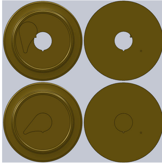
Figure 10. Front and back views of the eyepiece and cover in opened and closed configurations.
