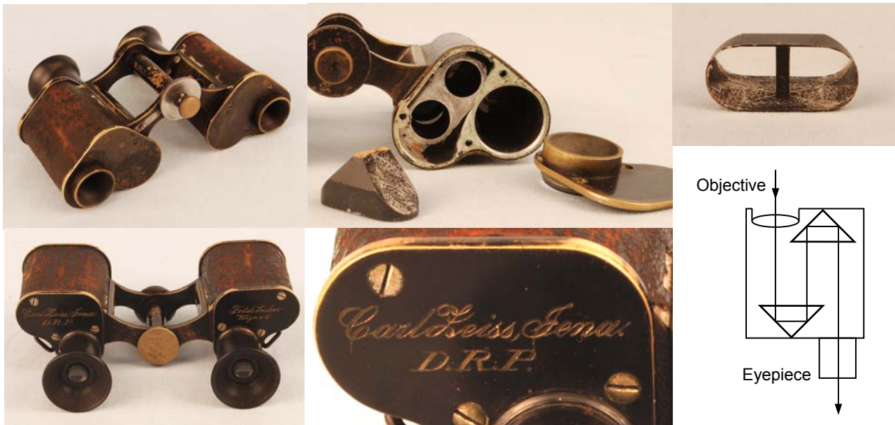
Figure 15. Zeiss 6X15 binoculars with serial number 306 (1895). The script inscription reads “Carl Zeiss, Jena D.R.P.” and “Feldstecher Vergr = 6”. The familiar Zeiss lens logo was first used in 1904. Removing the prism cover and the objective lens shows the prism mount and a Porro prism for a pair of 8X20 binoculars of the same era (No. 4976; 1897). The insert schematically shows the arrangement of the prisms in the housing. Of course, both prisms are actually rotated by 45 deg out of the plane. In this 8X pair, the prism separation is approximately 30 mm; the separation is approximately 20 mm in the 6X binoculars as the prism body is shorter.
