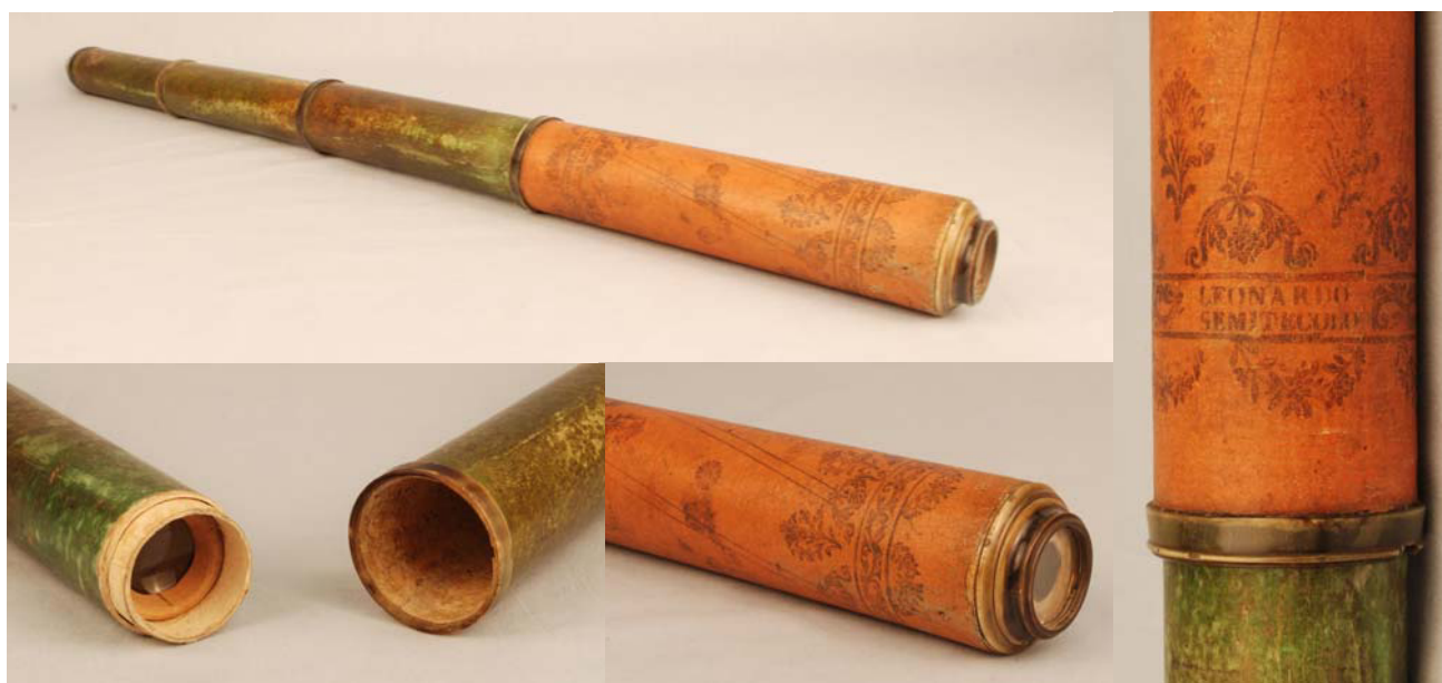
Figure 2. Italian 3-draw telescope by Leonardo Semitecolo (Venice) from the early 1700s. The telescope consists of cardboard tubes covered in decorated vellum. It is 850 mm in length and the main barrel is 55 mm in diameter. The objective lens diameter is 35 mm, and as was usual in pre-achromatic telescopes, a small aperture of 20 mm diameter is placed behind the lens to control longitudinal chromatic aberration. A Schyrle erecting system is used. The fittings on the tubes are horn with wood lens mounts.
