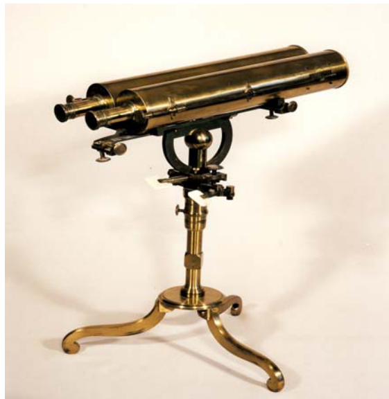
Figure 11. Gregorian reflecting binoculars (James Short, London, circa 1760). From the collection of Rolf Willach (Taegerwilten, Switzerland); photograph used with permission.
