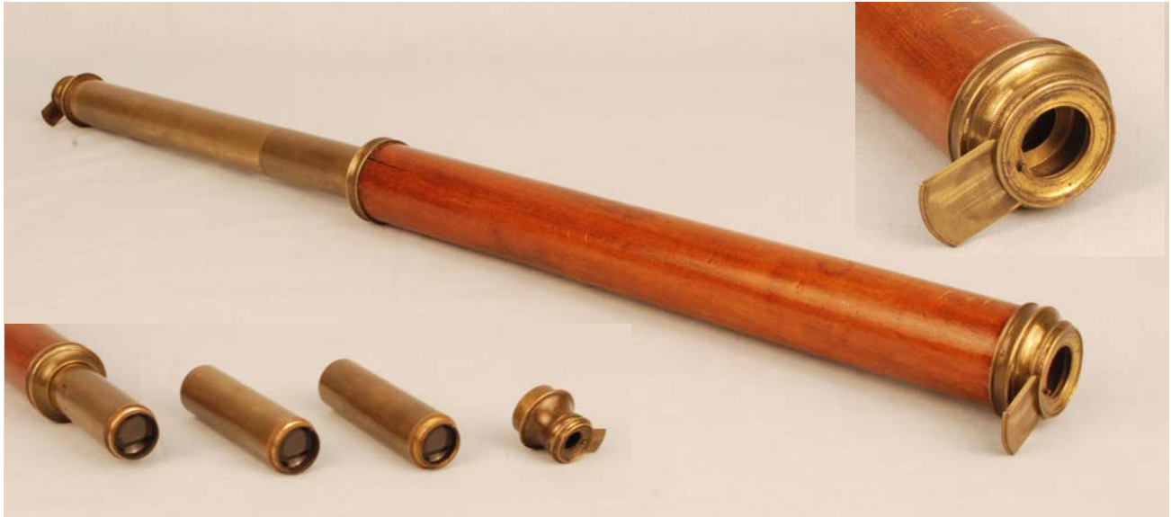
Figure 3. Single-draw pre-achromatic telescope with a wooden barrel and a Schyrle erecting system (unsigned, circa 1750, English). The telescope has an overall length of 570 mm. The objective diameter is 23 mm with a 13 mm diameter aperture. Each section of the draw contains one of the three lenses of the Schyrle erecting system.
