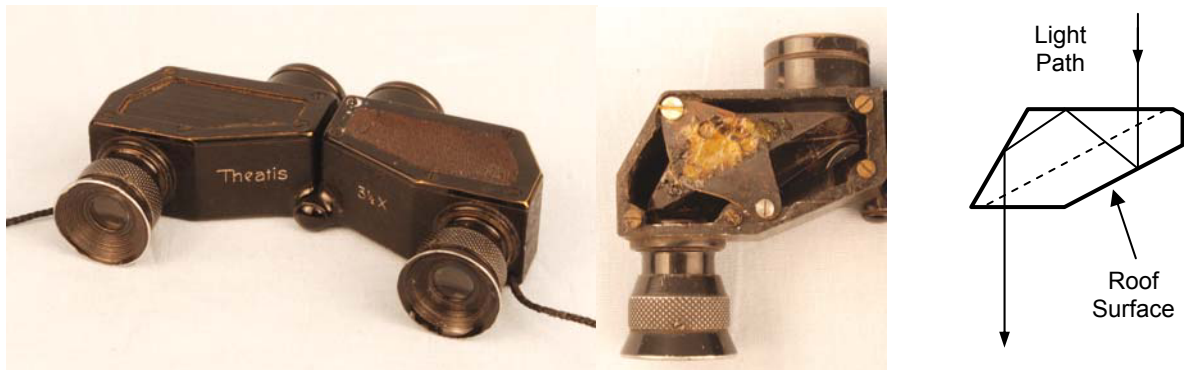
Figure 16. Leman prism binoculars (Theatis 3½X; J.D. Möller, Wedel, Germany, late 1920s). Four reflections are obtained with this compact image-erection prism.
