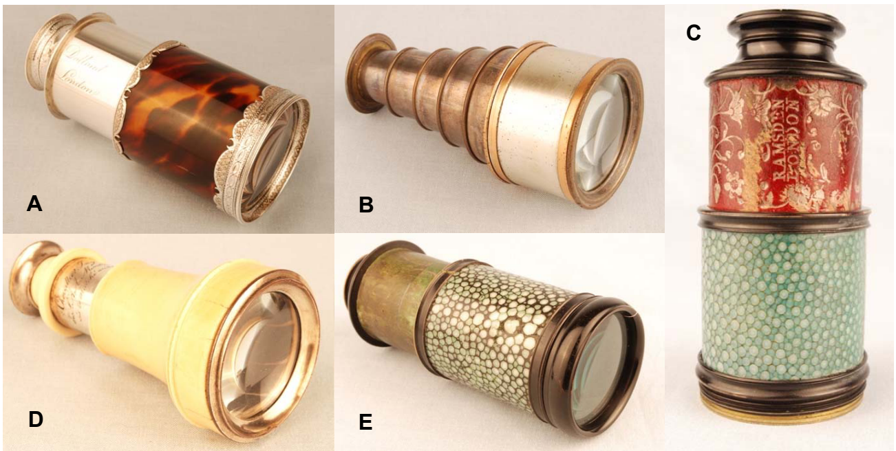
Figure 4. Galilean spyglasses: (A) Tooled silver and tortoise shell (Dollond, London); (B) Five-draw with silver plating (Dollond, London); (C) Cardboard draw with tooled leather, barrel covered with shagreen (Ramsden, London); (D) Ivory and silver-plated brass (Chevellier, Paris); (E) Shagreen covered wooden barrel with cardboard draw (Ayscough, London). All date from mid to late 1700s.
