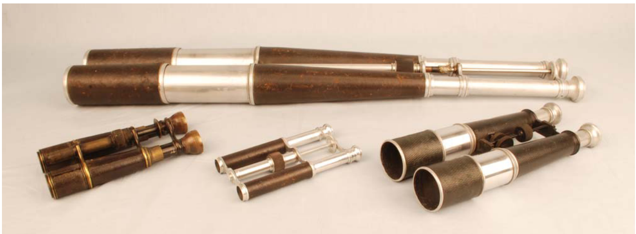
Figure 12. Various twin telescopes. All date from the late 1800s. Three of the twin telescopes shown are aluminum and one is brass. The large telescope has a length of 750 mm with its sunshades extended. The magnifying powers range from about 5X to 20X.
