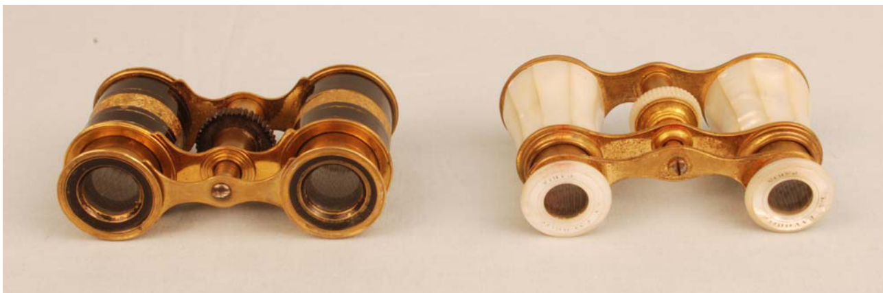
Figure 6. Opera glasses showing the two varieties of bridging frames. Both use a central knob that drives a third bridge for focusing (unsigned, French, mid-1800s; La Favorite, Paris, late 1800s).
