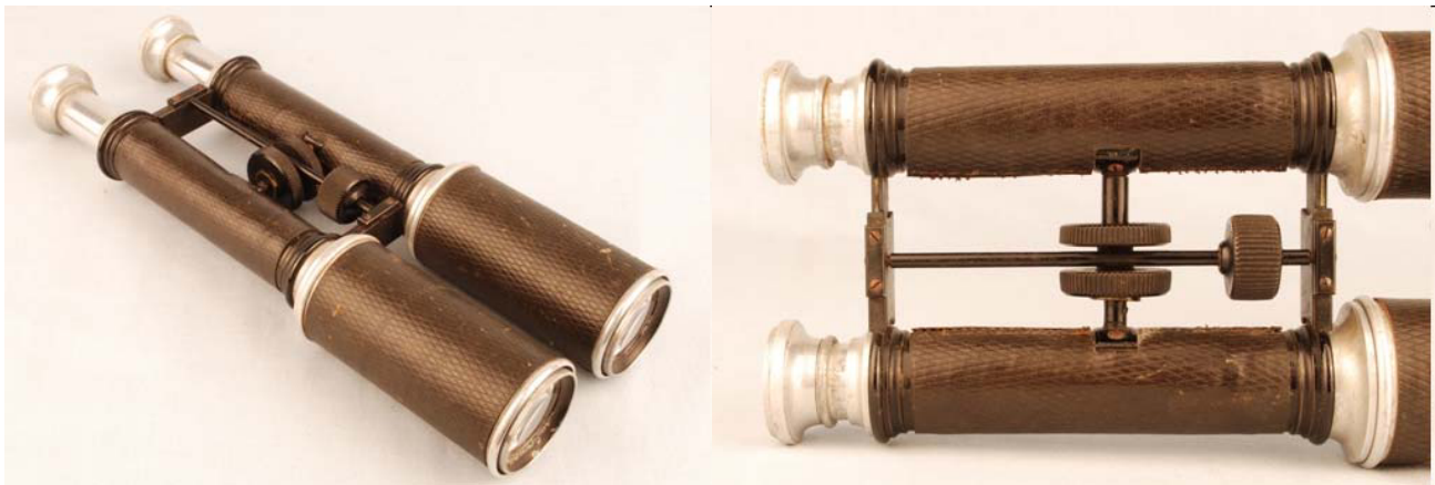
Figure 14. Twin telescope binoculars featuring rack-and-pinion adjustment of the interpupillary distance (Negretti & Zambra, London, late 1800s). The pair of knobs attached to the rod that is perpendicular to the telescopes adjusts the focus; the single knob adjusts the interpupillary distance.
