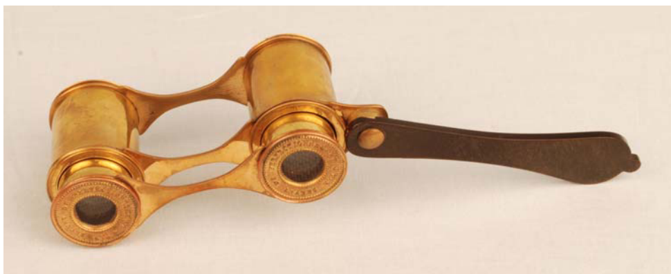
Figure 5. Lorgnette-style opera glasses with the early focusing mechanism. The left barrel is rotated to focus both telescopes, and the two eyepieces are attached to a third bridge. (French, early 1800s). The eyepiece inscription reads “Par Brevet de Perfectionnement,” indicating that this design is “by patent of improvement.”
