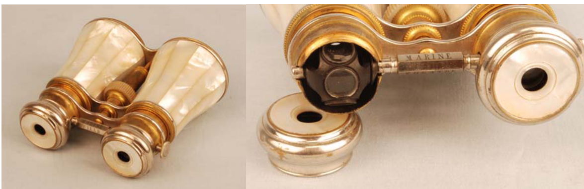
Figure 9. Triple eyepiece opera glasses (French, late 1800s). A knob on the side rotates turrets in both eyepieces to bring one of three different eye lens into place to achieve three different magnifications: Theatre ~2.5X; Field ~3X; Marine ~4X.
